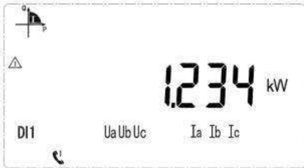
Current total power is 1.234kW
