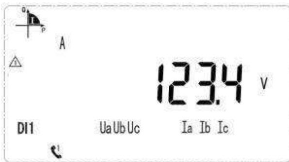
Voltage on A phase is 123.4V
