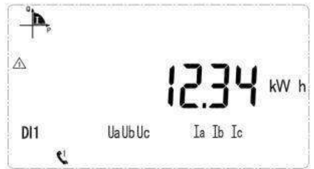
Current reversing active energy 12.34kWh
