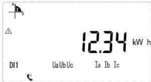
Current forward active energy 12.34kWh
