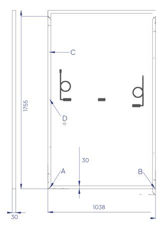
A: Drainage; B: Ventilation; C: Mounting holes; D: Earthing;
