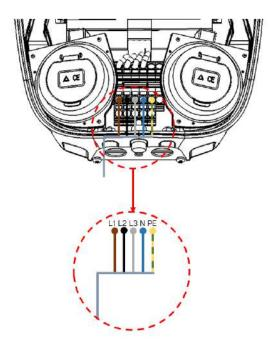
Note that if the power is to be routed onwards, connect the cable to be routed onwards to the other input on the terminals.
