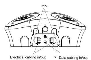
6. Mount Aura on the wall: Use the key supplied to unlock the cylinder lock underneath Aura. Rotate up and suspend the front. Align Aura on the wall according to the specified hole pattern. Make sure that the mounting has fixed Aura in place.
