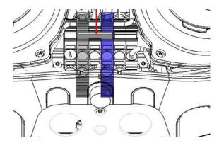
9. When the incoming cabling is installed, make sure that it does not arch over the dotted red line as illustrated below.
