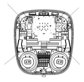
7. Connecting the electrics: Pull the power cable through the cable slide approx. 80 mm. Use a cable stripper to strip approx. 20 mm off the end of the conductors. Connect the conductors (L1–L3, N and PE) to the terminals.
