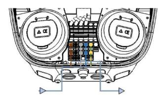
8. If you are installing Aura in an IT network, connect phase cables L1 and L3, and use 1–3 terminal blocks, which are included in the kit, as illustrated below. L2 and N will be connected together.
