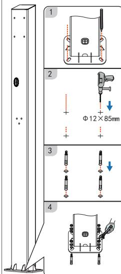
③ Install the backplate and the socket-out.
