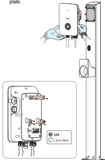
Pile installation effect diagram.
